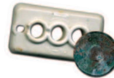
FOUND DURING CLEANING: PERIOD PORCELAIN WIRING ROUTER AND ALCOHOLICS ANONYMOUS MEDALLION
