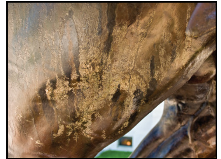
FLAKING WAX IN 2007 COVERS NEARLY 40% OF THE GENERAL JOHN F. HARTRANFT STATUE.
